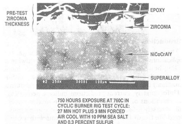
Fig. 3 Sulfate salt films wicking into the microstructure damage columnar-grained EB-PVD zirconia coatings
