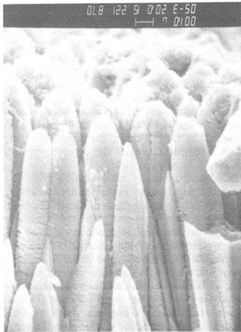
Fig. 5 Electrical biasing produced a thin, dense surface layer that bridged the intercolumnar porosity of the EB-PVD ZrO 2
