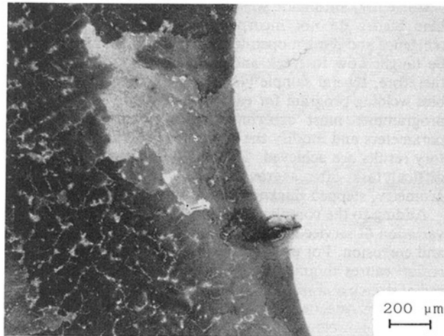
Fig. 2 Typical acceptable defects in a turbine blade (alloy: B1900)
