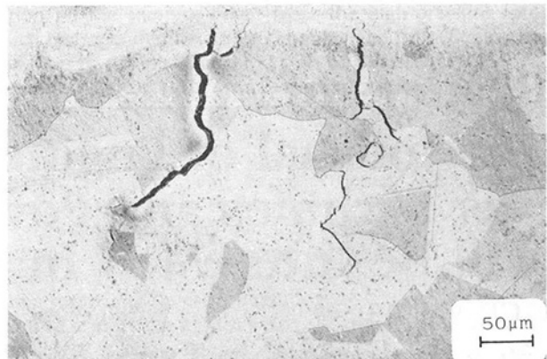
Fig. 1 Micrograph showing typical HAZ microcracking in a superalloy weldment (alloy: IN738LC)
